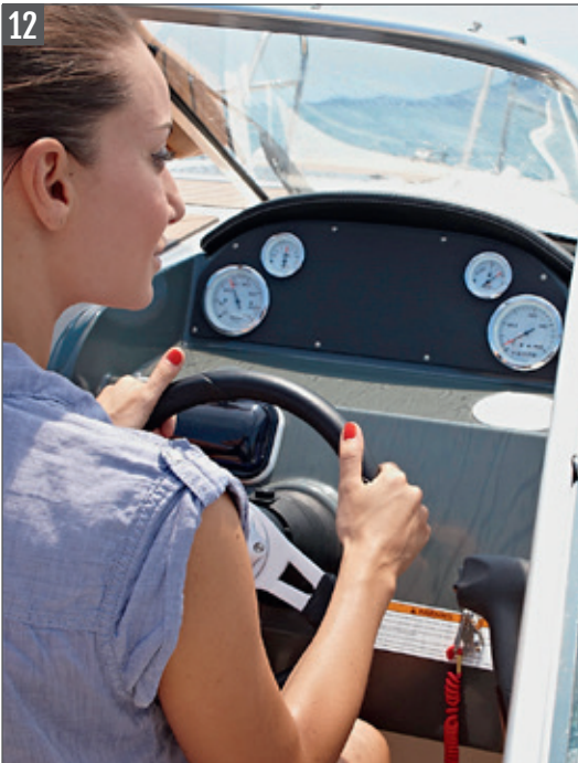
Integrated helm with hydraulic steering, SmartCraft instrumentation, mounting area for 7" GPS/Chart Plotter and 12v outlet
