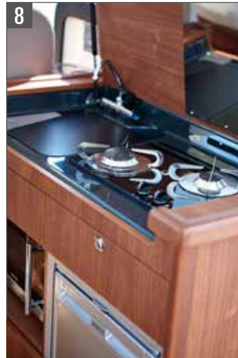
Galley with pressure water, LPG stove, refrigerator and microwave
